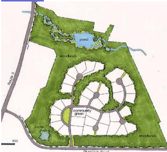
The key ingredient in conservation subdivisions is open space surrounding residential lots.
